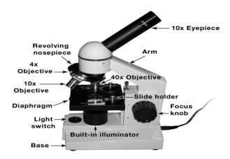
Look at the picture above. Each of the parts of the microscope is labeled. The major parts of the microscope are the light source, the specimen stage, the eye piece, and the objective lenses. You will find a description of the microscope parts at the end of this write up.
