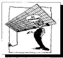
nected directly to the AC line. The utility may require a second meter and disconnect. The installation cost of this type of intertie system is much lower than that of a large inverter system. A small system can be installed, and as finances allow, additional AC PV modules can be easily added to the system.
